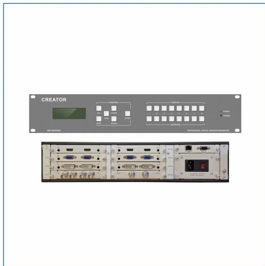
CR-MID MAX0808 Size (mm): 483(W)x365(D)x89(H)
